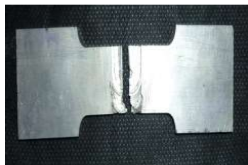
Fig 1.7: Tensile test specimen after test
