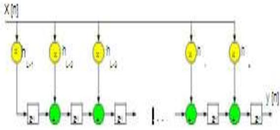
Fig. 1. A MAC FIR filter block diagram.
