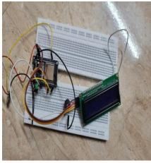
The prototype system underwent initial testing using both simulated pulse signals and real-time data from human subjects under controlled conditions. The system demonstrated the ability to accurately track pulse rate values within a range of 55 to 120 BPM. The anomaly detection mechanism effectively triggered alerts when the simulated or measured BPM fell outside the predefined thresholds (below 60 or above 100 BPM). The real-
